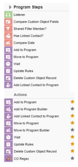
• Drag and drop the cloud action to the canvas area. Connect the corresponding elements to the dropped cloud action
